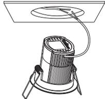
2. Connect the brown (L) & blue (N) input wire of power supply to live line & zero line. (Off-power operation)
