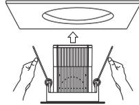
3. Push springs of light as vertical and embedded lamp into the ceiling.
